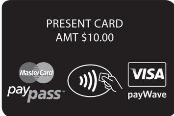
Tap, Insert or Swipe cardholder's card. Chip Cards are to be inserted and left in the Chip Card Reader. Contactless Cards or smartphones are to be tapped on to the screen. Magnetic Stripe Cards are to be swiped through the Magnetic Card Reader.
