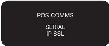
Press the down or up key to cycle between Serial and IP SSL, press ENTER on your selection.
