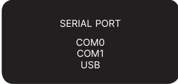
Press the down or up key to cycle between COM0 (for Serial), COM1 and USB (for USB), press ENTER on your selection.
