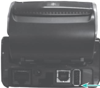
Connect the USB, Serial and Power cables into these ports
