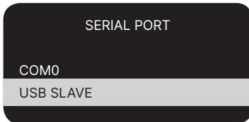
Press <▼> key or <▲> key to cycle between the COM0 and USB connections.
